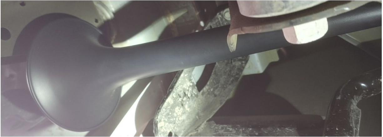
Figure 24- Trumpet Alignment to Prevent Vehicle Contact
