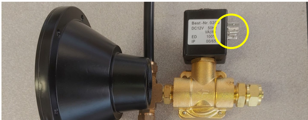
Figure 8- Solenoid Electrical Connector Removal
