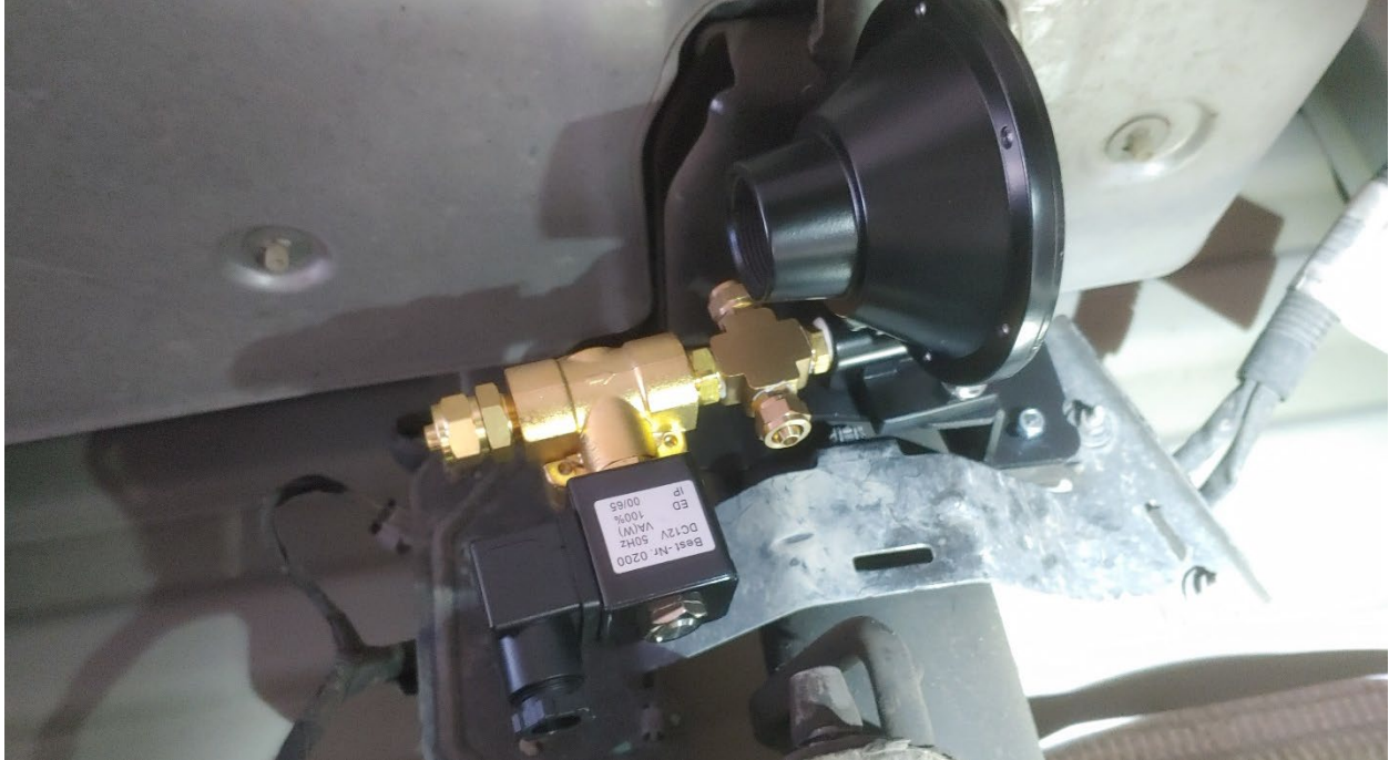
Figure 28- Center Air Horn Bracket & Driver Temporarily Attached (Shown Without Air Tubing for Clarity)
