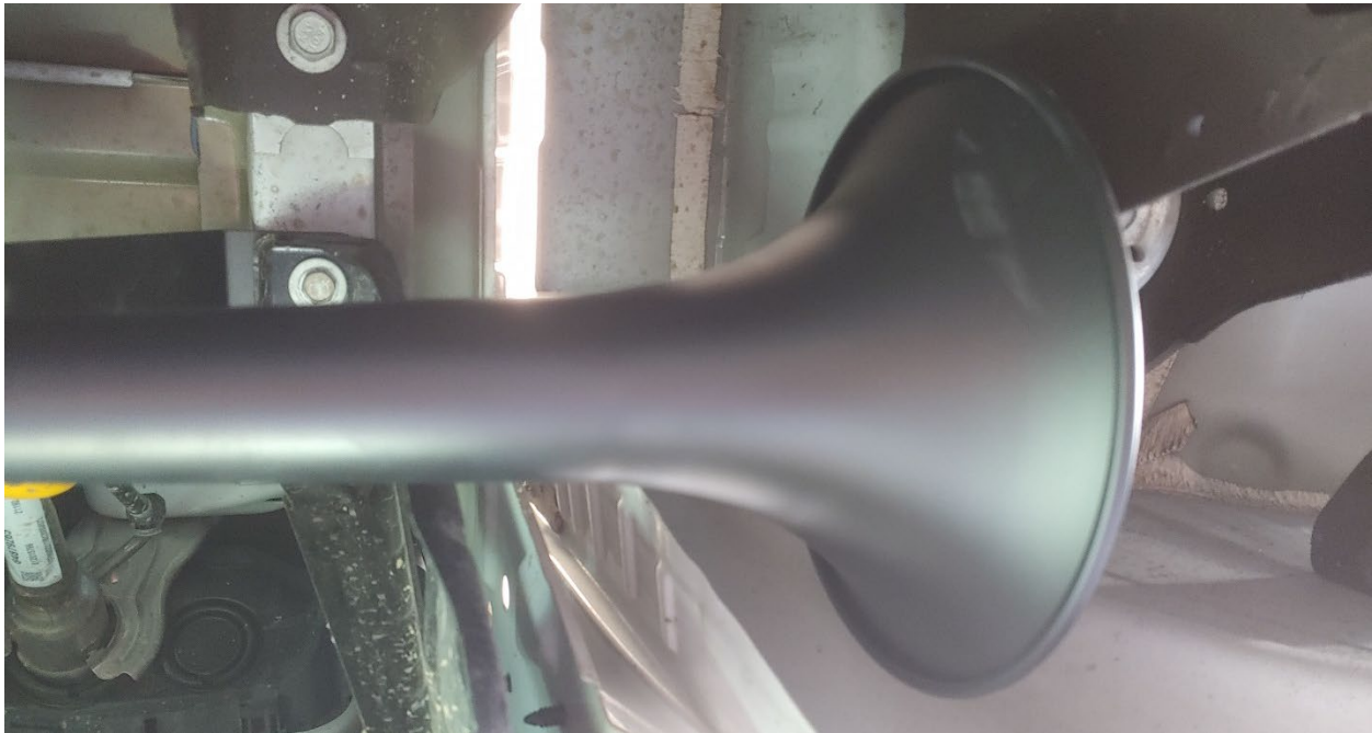
Figure 19- Trumpet Alignment to Prevent Vehicle Contact
