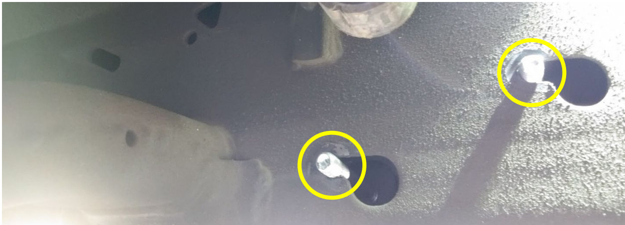
Figure 34- Compressor Bracket Installation, Inside Frame Rail
