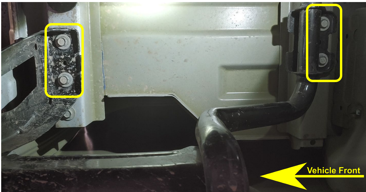
Figure 22- Passenger Side Horn Bracket, Mounting Points
