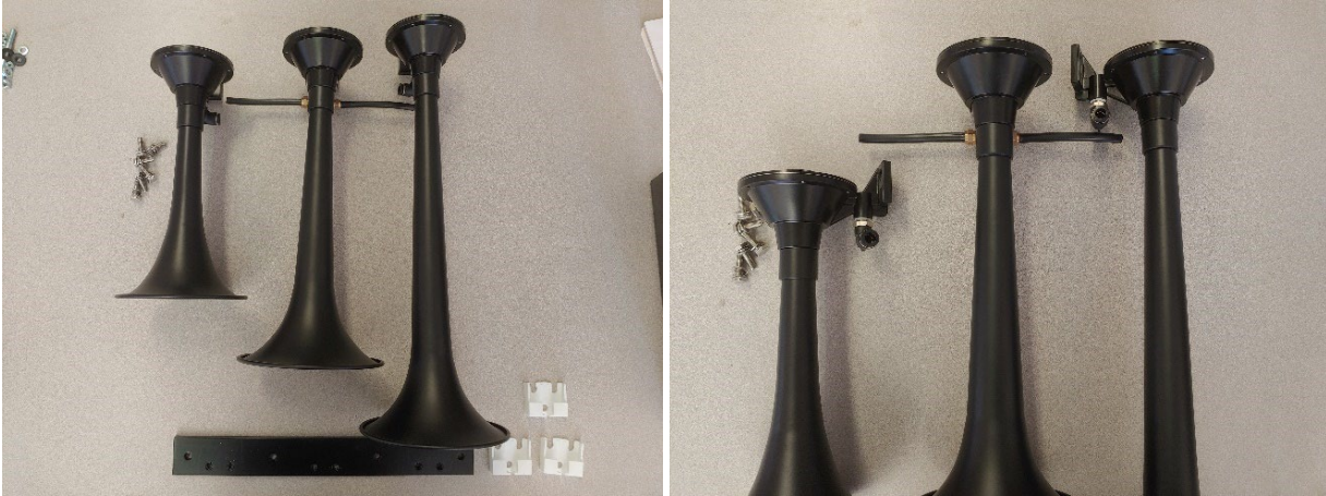
Figure 5- Air Horn Disassembly & Separation
